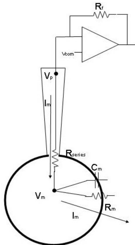
tip and the interior of the cell. Series resistance adds two types of errors in patch clamping:
