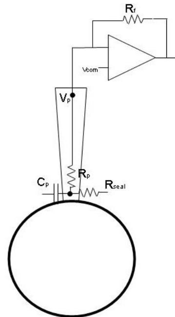
the signal as a low pass filter with a time constant,  $\tau_p = R_p C_p$ .
